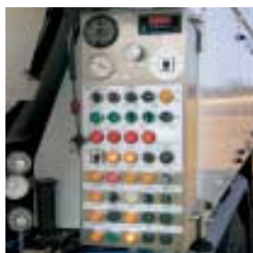
Control panel from which a simple and userfriendly control of the vehicle is carried out. The control panel is made of stainless steel.
