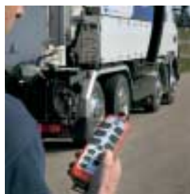
Remote control is normally delivered with 8 eligible functions and may be extended with 3 extra functions. (The remote control is extra equipment).
